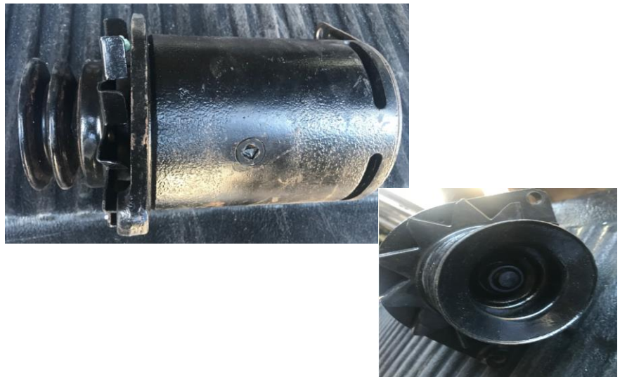
Ford generator FAS10139B; dual belt; appears to be rebuilt
