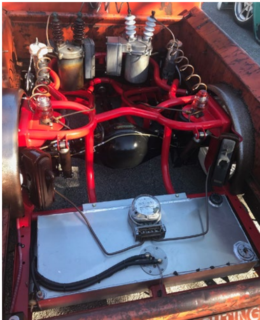
L.I.L.C.O. is Long Island Lighting Co. I remember the Utility trucks all over when I was a kid. They never looked like this. Notice the Air suspension components disguised as transformers and a utility meter!
