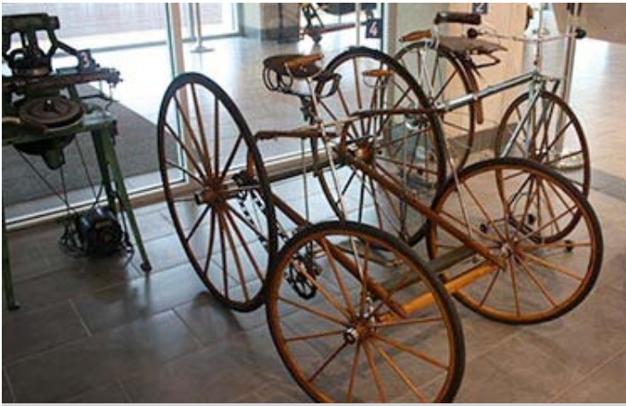
Quadracycle with the steering knuckle invented by Sterling Elliott
