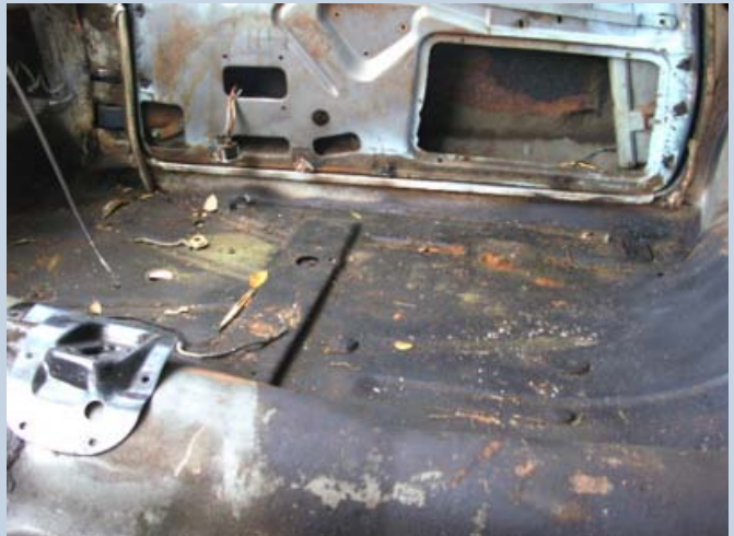
floor has been cleaned and rubberized
