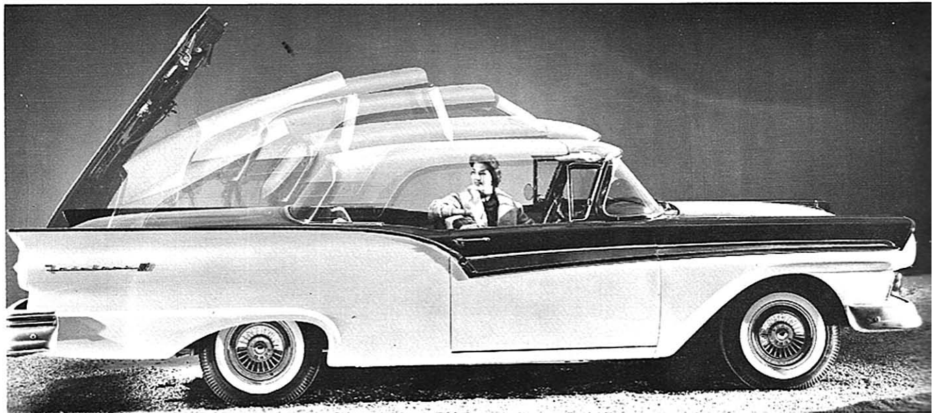
Ford's production fliptop used 13 switches, 9 circuit breakers, 5 motors, 610 feet of wire. Rear of body stands higher than conventional 1957 models.
