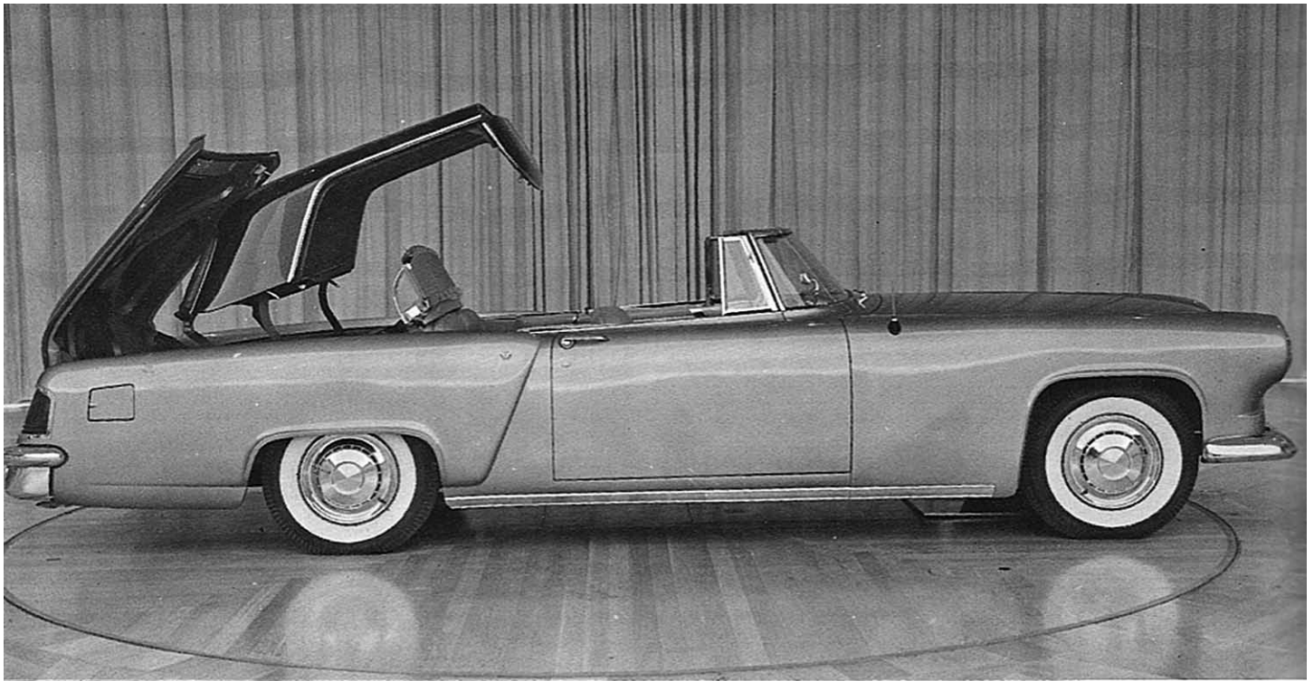
First Ford product to get fliptop was this Continental Mk. II prototype. When Continental Div. decided not to build retrac, development
